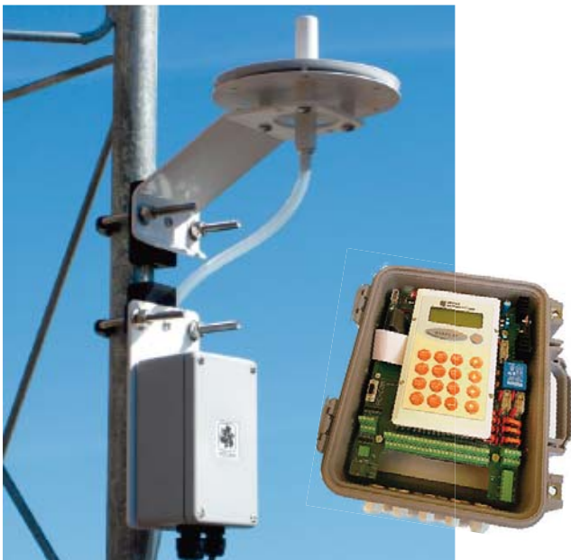
Weatherproof Enclosure and Pressure Port and Datalogger
